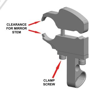
STEP 3 - BEFORE FULLY TIGHTENING THE CLAMP SCREW, POSITION THE MOUNT AS FAR FORWARD TO-WARDS THE WINDSHIELD AS YOU CAN. MAKE SURE THE TOP AND MID SECTIONS ARE TOUCHING AT THE PIVOT POINT. If you can not get them to touch at the pivot point, you have an incompatible mirror type for this mount.
