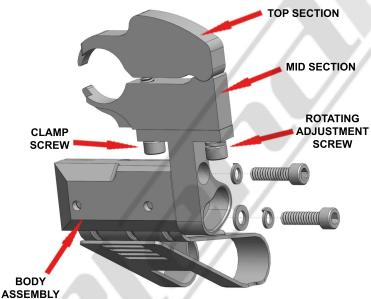
STEP 2 - The BODY ASSEMBLY must be removed to gain access to the CLAMP SCREW. Remove the two socket head screws as shown above. Be sure to remove the lock washer with the top screw along with the lock washer and flat washer with the bottom screw. Loosen the CLAMP SCREW so there is enough clearance between the TOP and MID SECTIONS to slide over the mirror stem. YOU MAY ADJUST THE MIRROR PARALELL TO THE WINDSHIELD AND SLIGHTLY UPWARD FOR EASE OF INSTALLATION.
